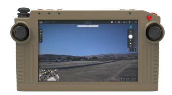
Universal mobile GCS for UxS operators, with daylight readable screen, onboard GPS, interchangeable radios, and multiple control applications to meet different user demands.
