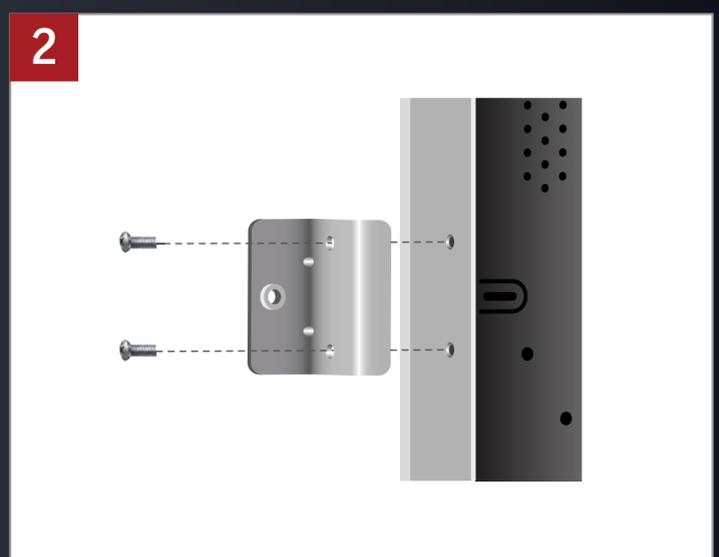
2 Place the mounting bracket to the UPC and fasten it, tighten each mounting bracket on every side
