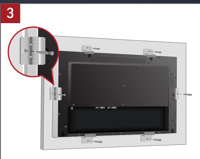
3 Fasten the screw to fix the bracket to the panel
